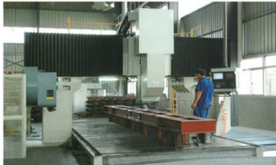
CNC gantry pentahedron machining center. This machining center can process 5 surfaces of parts with once fixing and guarantee tolerance of every surface. What's more, with CNC four axis linkage. It is ideal for tubing drilling boring, arch machining and so on.
