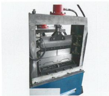
▶ 液压切断 Hydraulic cutting with waste
