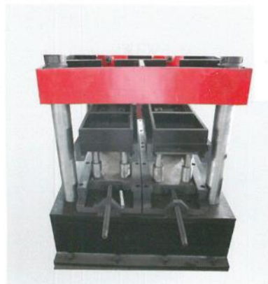
▶ 液压冲孔装置 Four column hydraulic punching device
